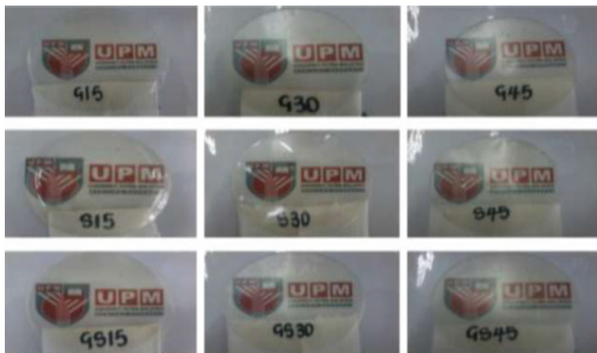
Fig. 7.10 SPS films prepared using different plasticizer type and concentration (Sanyang et al. 2016b)
