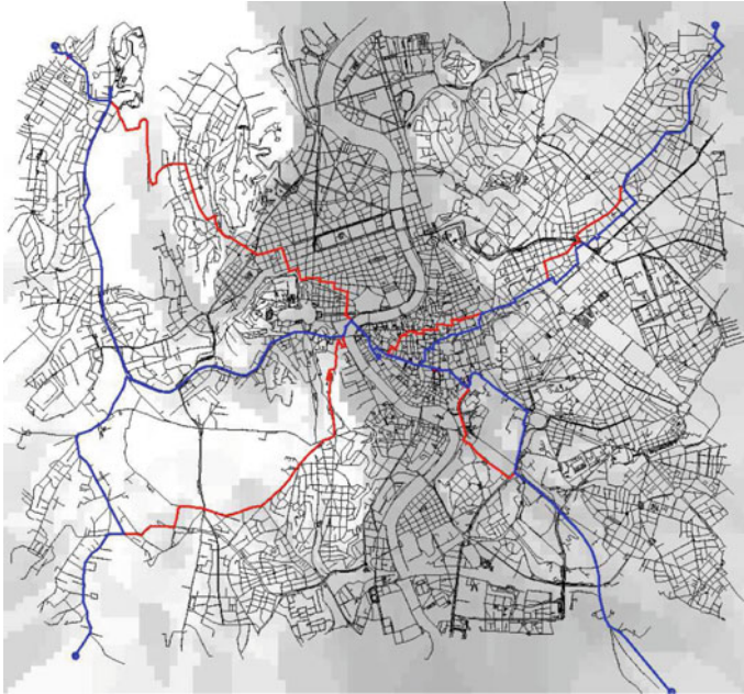
Fig. 4 Map of Rome. The altitude is shown by the background color (highest is brighter). The map shows eight paths starting from the center to the four corners. In red the shortest paths, in blue the paths produced by our MIP model
