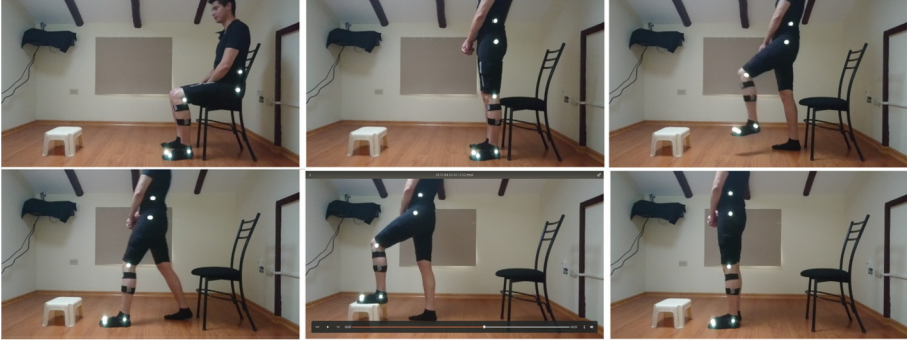
Fig. 5. Sequence of movements (trial) defined to compute the joint angle in sagittal plane using Optical and our fused motion capture. Figure illustrates sequence of movements, which can be viewed from top-left to right frames
