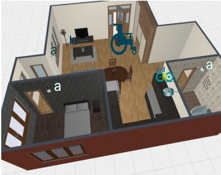
Fig. 2. Sensors distribution within the house.
