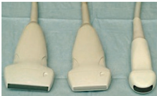
FIGURE 12.2 From left to right demonstrates different footprint sizes, linear array transducers with the transducer on the right demonstrating a smaller, curvilinear array transducer)
