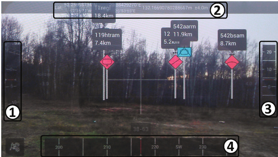
Fig. 6. AR based situation awareness view merging sensor data, battlespace information and threat level estimates (1 – deflection, 2 – location, 3 – elevation, 4 – azimuth)
