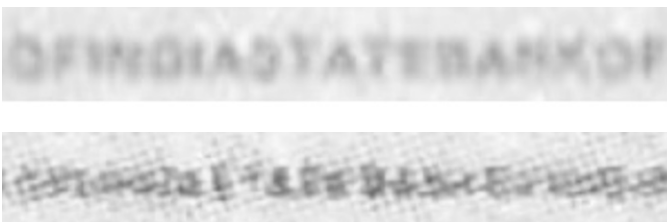
Figure 5. Zoomed views of microlines on genuine (top) and printed checks (bottom).
