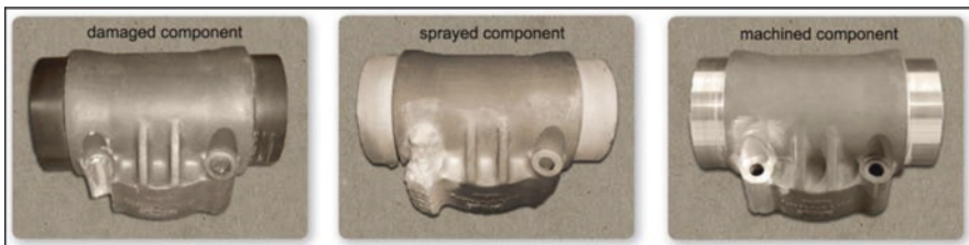
Fig. 6.11 CSR process of a mechanically damaged flap transmission tee box housing of an aircraft (Schell 2016)
