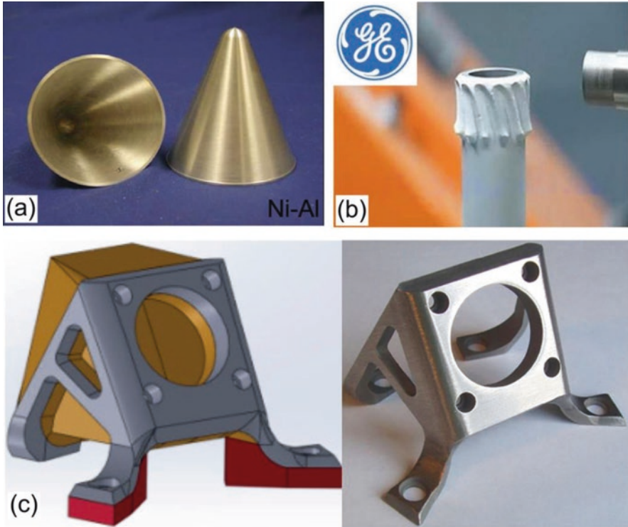
Fig. 6.6 Digital photos of CSAM components with complex structure: (a) cone structure, (b) gear, and (c) bracket (Briefing 2013; Champagne and Helfrich 2016; Richter 2014)
