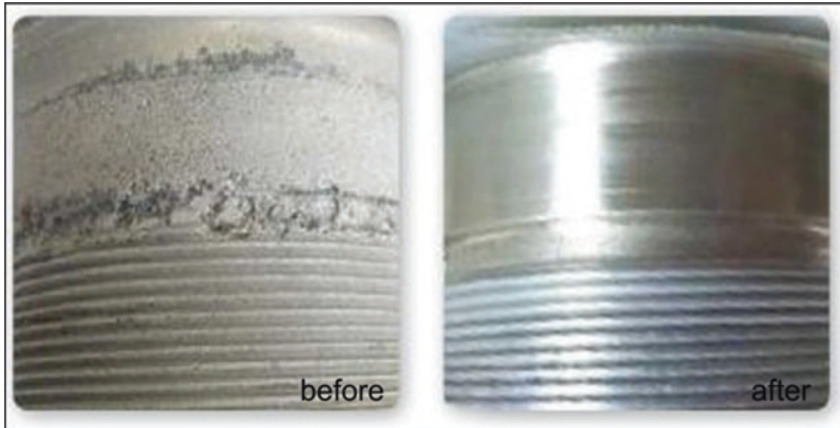
Fig. 6.10 Restored B737 nose wheel steering actuator barrel via CSR (Schell 2016)
