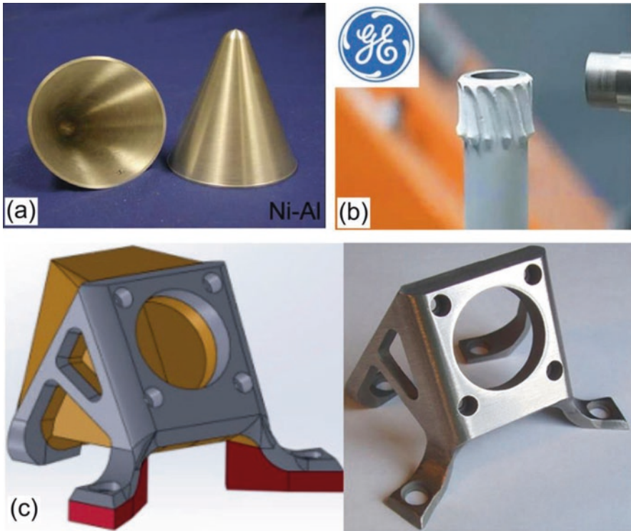
Fig. 6.6 Digital photos of CSAM components with complex structure: (a) cone structure, (b) gear, and (c) bracket (Briefing 2013; Champagne and Helfrich 2016; Richter 2014)
