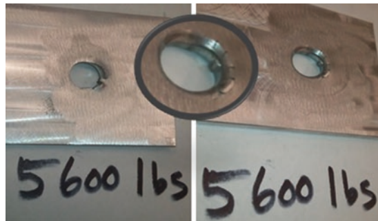
Fig. 2.12 Test coupon with a fastener installed into a hole repaired by cold spray and inserted into a test fixture designed to test the cold spray repair simulating an actual FEB panel
