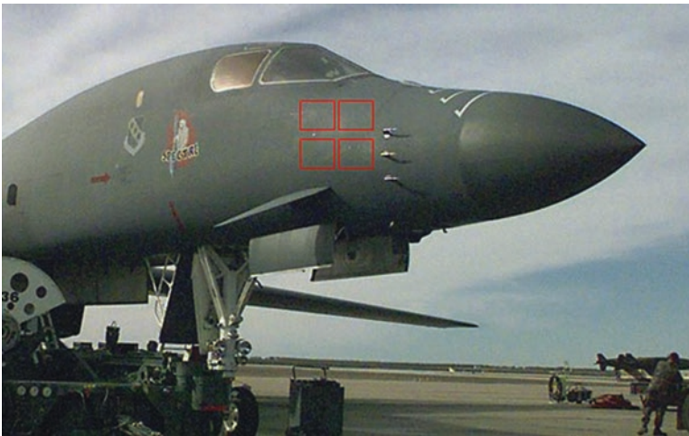
Fig. 2.8 Forward equipment bay (FEB) panels on the B-1 Bomber repaired 2012
