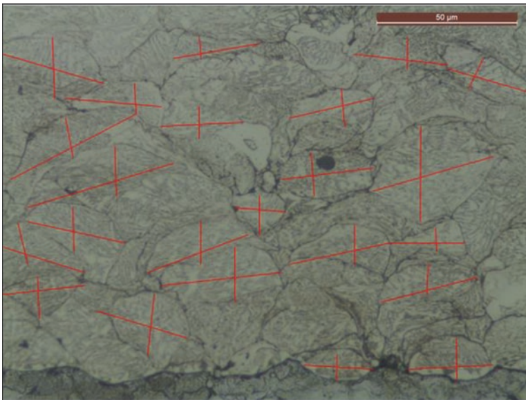
Fig. 17.1 Example of splatted cold spray particles
