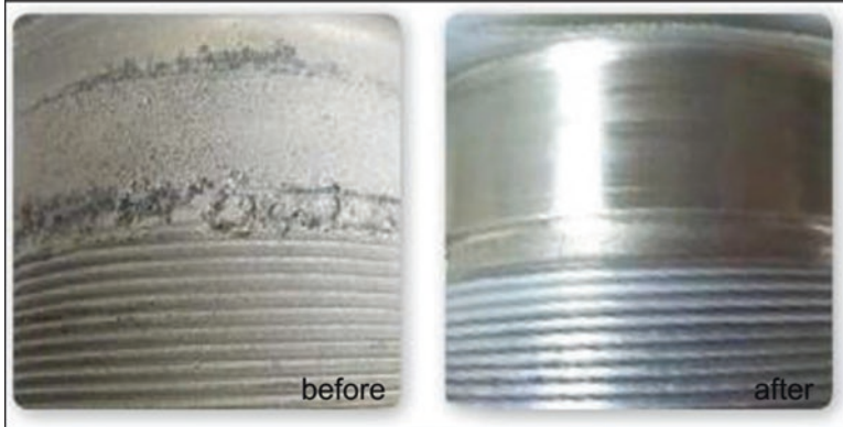
Fig. 6.10 Restored B737 nose wheel steering actuator barrel via CSR (Schell 2016)
