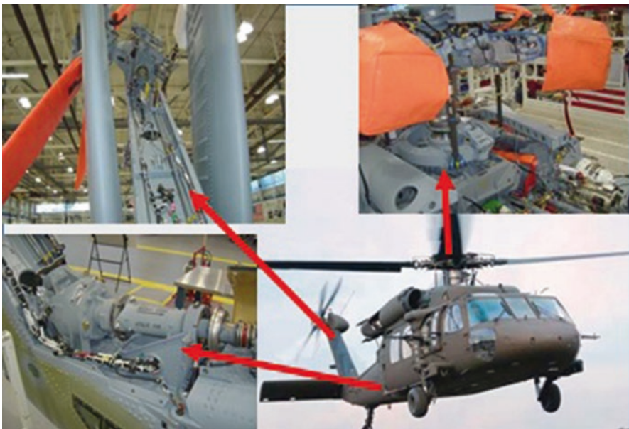
Fig. 2.1 Corrosion-prone areas on UH-60 Black Hawk transmission components
