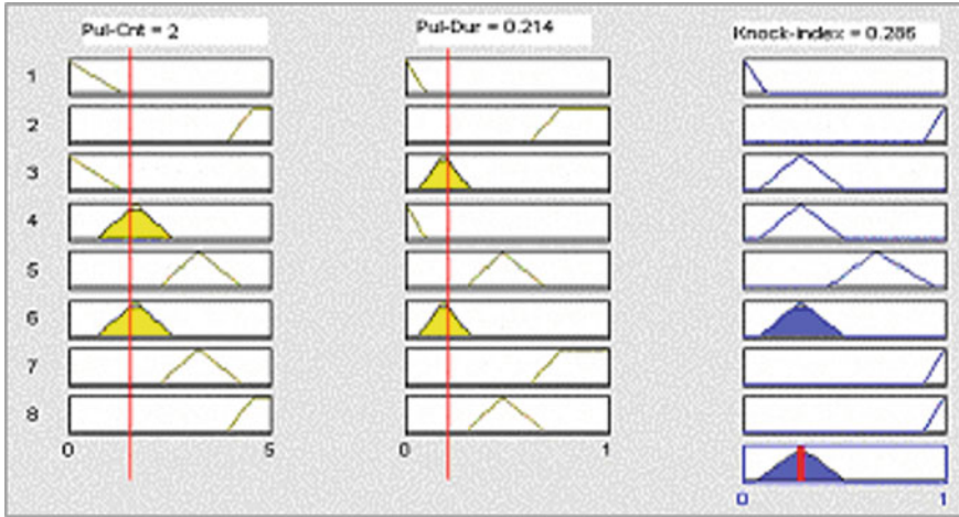
Fig. 5.10 Values of Knock Index for each couple of inputs ( Pul_Cnt and Pul_Dur )
