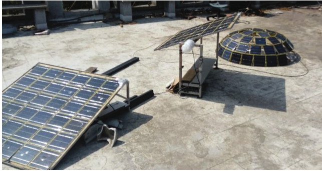
Fig. 1. Experimental setup – (a) Fixed panel, (b) Single axis STS and (c) Dome structure
