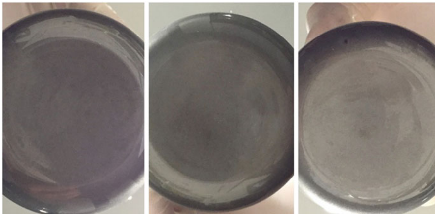
Fig. 7.14 The bottom of the jar when mixing the dye with 0.2 wt% of \text{Fe}_3\text{O}_4 . Left , 10 min. Centre , 20 min. Right , 30 min
