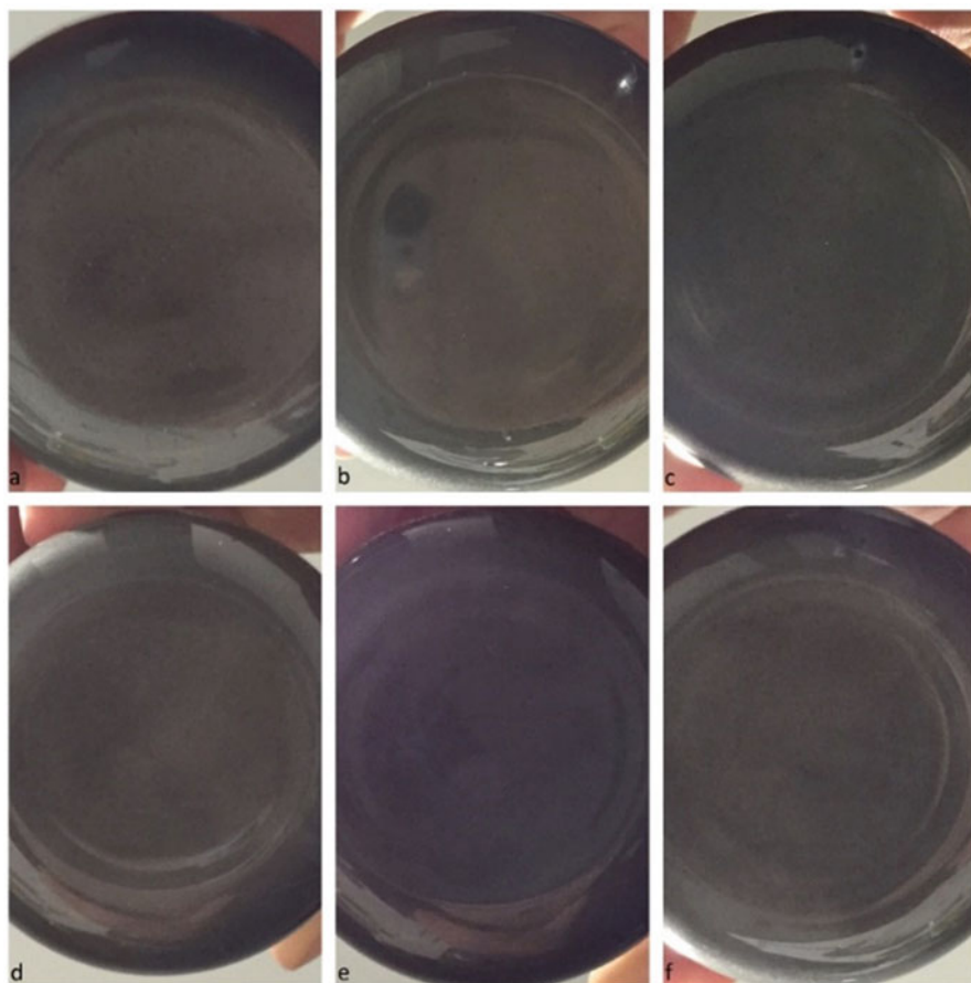
Fig. 7.11 Bottom of the jar of Sol1.2, while mixing manually with the glass stick and with the ultrasonic bath: (a) 5 min, (b) 10 min, (c) 15 min, (d) 20 min, (e) 25 min, (f) 30 min
