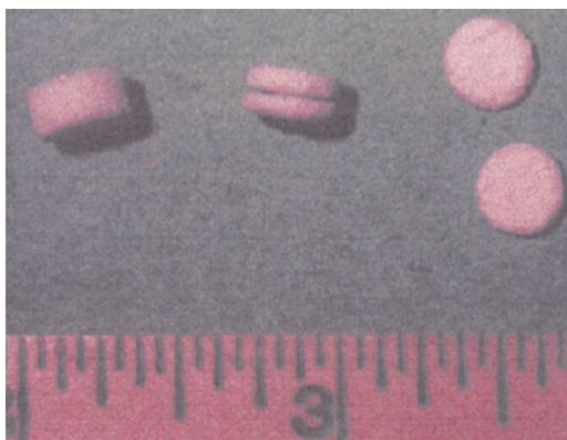
Fig. 16.9 Eudragit RLPO tablets before and after dissolution (Katstra, W.E., et al., Oral dosage forms fabricated by three dimensional printing. J Control Release , 2000, 66(1): p. 1–9.)
