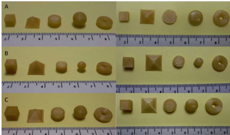
Fig. 16.23 3D printed tablets with different geometries at constant (a) surface area, (b) surface area/volume ratio and (c) mass (scale bar in cm) (Goyanes, A., et al., Effect of geometry on drug release from 3D printed tablets. Int J Pharm, 2015. 494(2): p. 657–663.)
