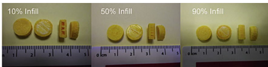
Fig. 16.21 Images of 3D printed tablets with different infill percentages (Goyanes, A., et al., Fused-filament 3D printing (3DP) for fabrication of tablets. Int J Pharm , 2014. 476(1–2): p. 88–92.)
