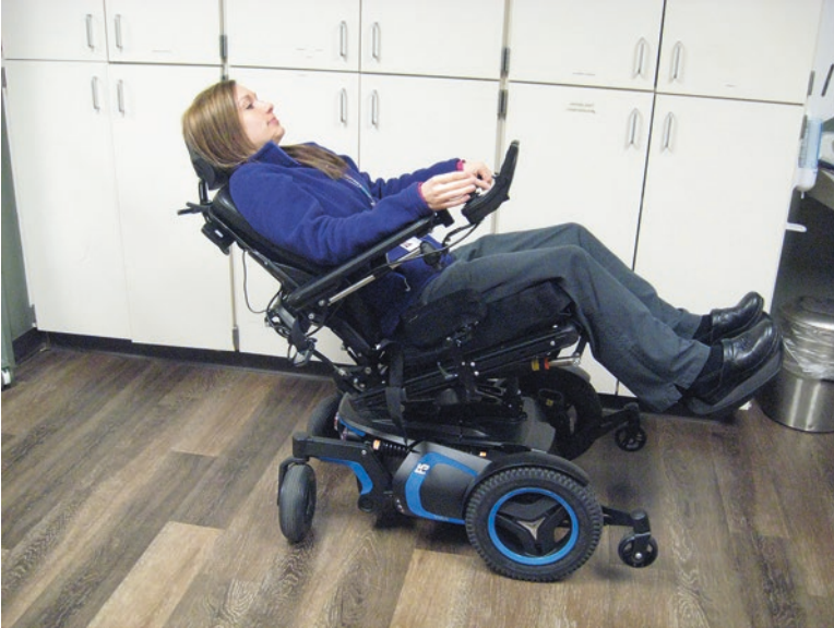
Fig. 7.2 Tilt-in-space option on front-wheel drive Permobil F5 power wheelchair™
