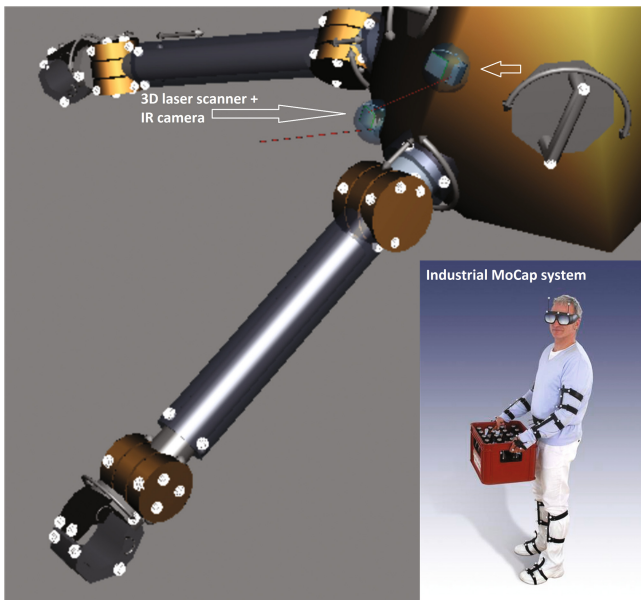
Fig. 5. The idea of the perception of partner robots by a bridge-robot is based on industrial MoCap systems, as given in the sub-photo in in the bottom right corner. The glass domes of two compound eyes are pointed to by white arrows. They can rotate in the eye sockets. Such an eye dome hosts laser 3D scanners (to scan ruins under and around the robot) and an IR camera for markers triangulation.
