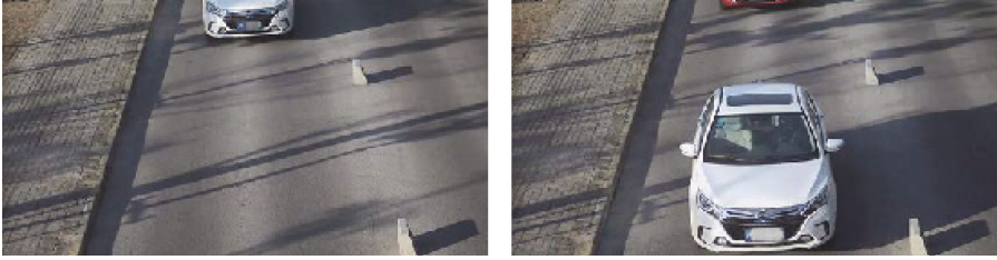
Fig. 2. The 1st frame (left) and the 26th (right) frame of vehicle images to calculate the transformation matrix.
