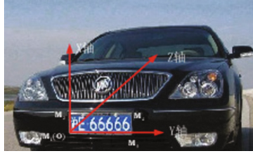
Fig. 1. The word coordinate system on the license plate.
