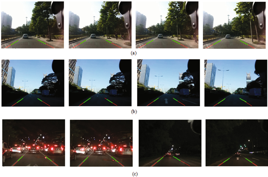
Fig. 2. Lane detection results in various illumination conditions: (a) front lighting, (b) back lighting, (c) night
