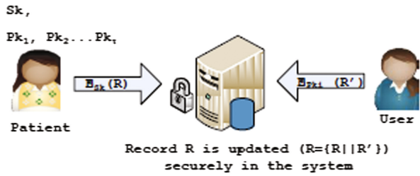
Fig. 1. A user can update a patients’ record in the secured server without knowing the content of the record
