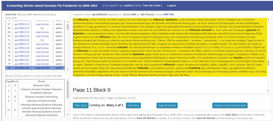
Fig. 2. Main GUI of our tool for extracting newspaper articles about the Russian flu from OCR text.
