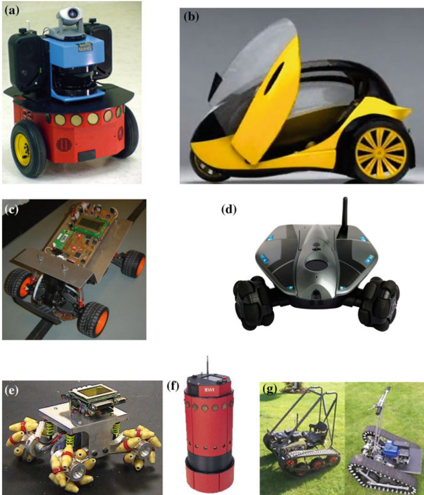
Fig. 12.19 Examples of mobile robots: a Pioneer-3 differential drive, b tricycle, c car-like, d omnidirectional/universal drive, e omnidirectional/mecanum drive, f omnidirectional/synchro drive, g skid steering/tracked robot
