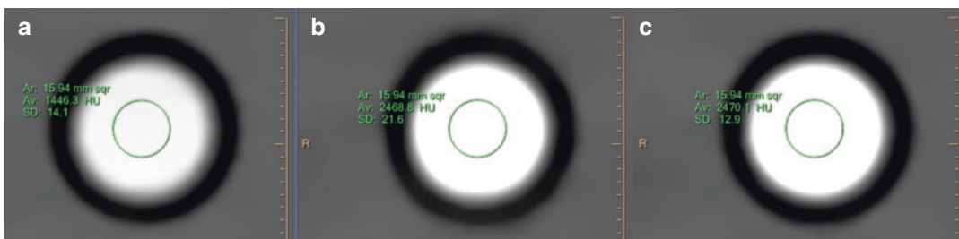
Fig. 14.4 Attenuation of iodinated contrast with different kilovoltage (a) 120 KVp image (HU) (b) 80 KVp image with higher attenuation and increased noise (SD)
