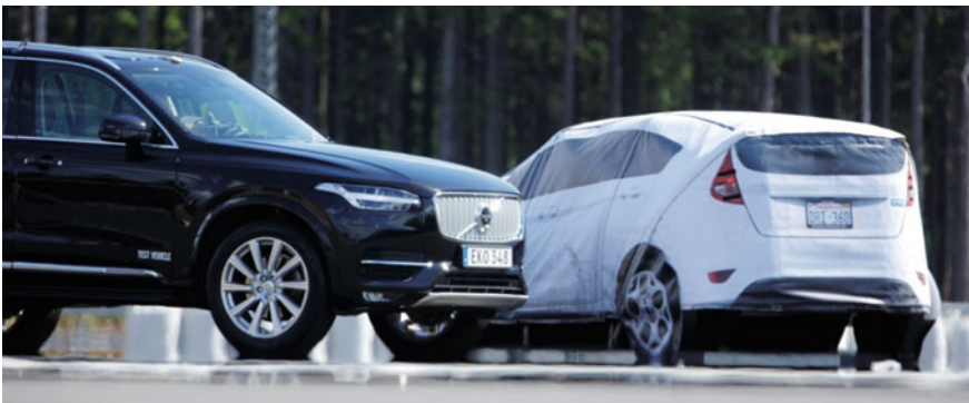
Fig. 1 Soft Car Targets (SCT) are used for safe and repeatable evaluation of ADAS and AD
