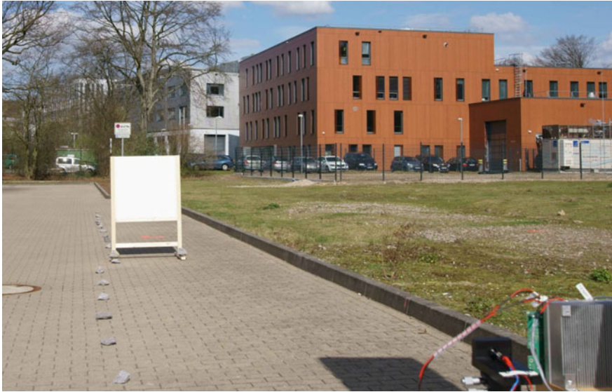
Fig. 3 Setup of the sensor range measurement at high ambient illumination. The target (e.g. white paper with 80% reflectance) is placed in increasing distance in front of the laser source and sensor. In this example an ambient illuminance of 90 klux was measured at the target surface
