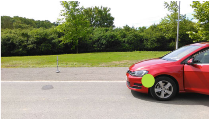
Fig. 1 Mounting position of side-looking radar sensors
