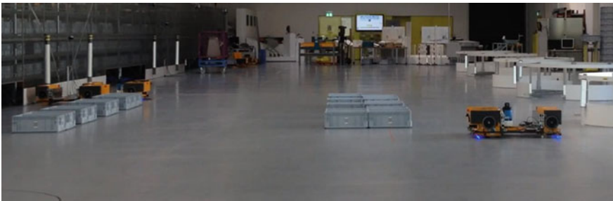
Fig. 1 Estimating the position of a free navigating AGV with limited height based on distance measurements is affected by changes in the environment (boxes in the open space)
