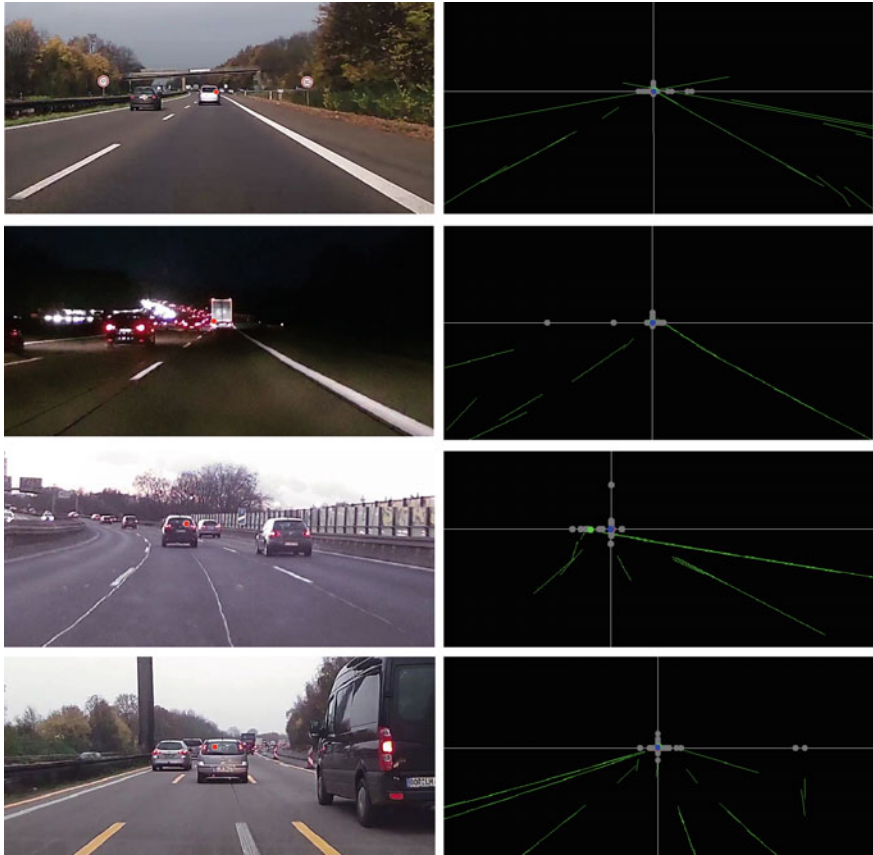
Fig. 7 Example frames from different test videos. It can be seen that the vanishing point is detected reliably across all frames. Left Input frames with detected vanishing points as red circles . Right Vanishing point estimation. Green lines represent simplified markings, the green dot is the estimated vanishing point, and the blue dot is the integrated vanishing point
