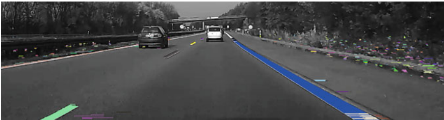
Fig. 5 Results of the double-edge grouping step. Each color represents a group of double-edge segments that likely belong to the same lane marking
