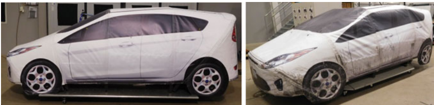
Fig. 2 The used SCTs, left is in near mint condition and right has been heavily used
