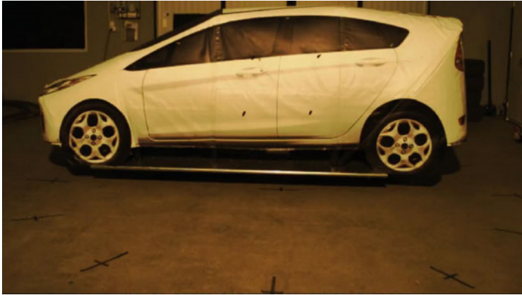
Fig. 3 Example of the image collected by the vehicle camera system. Four black pointers on the SCT side indicate the position of measurement spots for the spectroradiometer. Also visible on the floor are the markings for center position and rotation of the SCT
