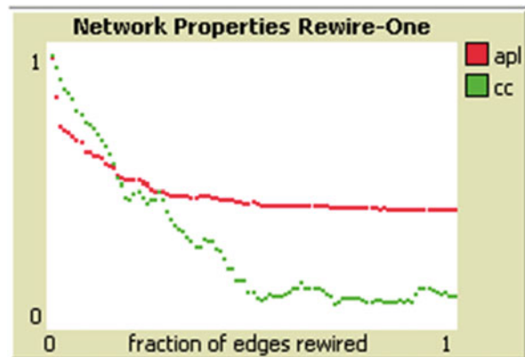
Fig. 19.7 Average path length (red) and clustering coefficient (green) represented as the probability of rewiring evolves
