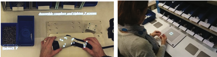
Fig. 1. Flexible operator support system with instruction projection.
