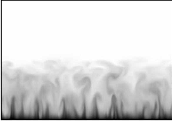
Fig. 1 Stream-wise velocity field from a numerical simulation of a turbulent flat-plate boundary layer flow at Re_{\theta,0} = 300
