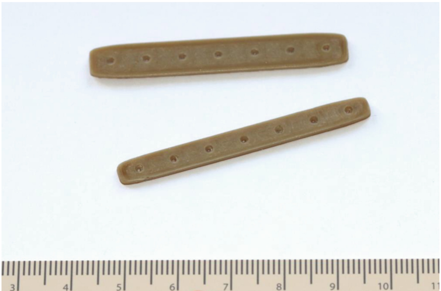
Fig. 1. 3D-printed PEEK osteosynthesis plates (length of 50 mm)
