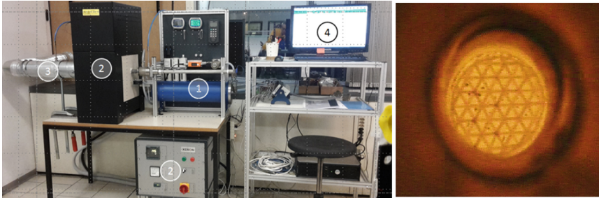
Fig. 3. On the left the test apparatus: (1) flow metering, (2) furnace, (3) exhaust, (4) control unit. On the right a ceramic architecture during high temperature test (700 °C)
