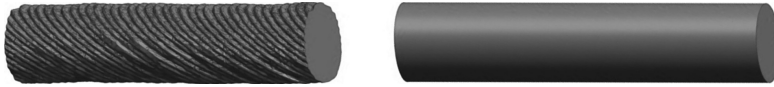
Fig. 2. 3D printed strut compared with a theoretical strut: on the left a strut surface reconstructed from CT micro tomography (source EMPA), on the right the surface of the corresponding strut realized by CAD.
