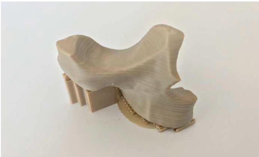
Fig. 3. Exactly fitting 3D-printed lightweight PEEK implant for immediate replacement of the zygomatic bone after tumor surgery
