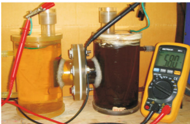
Fig. 11.3 Schematic details and photograph of H-type dual chambered MFC (Venkata Mohan et al. 2008)
