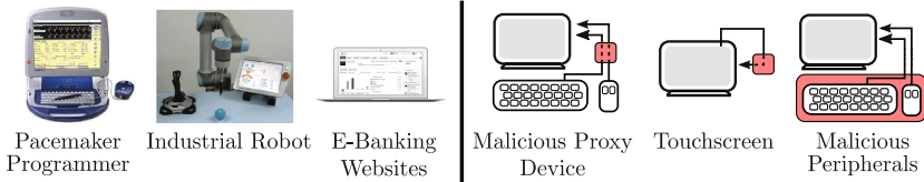
Fig. 1. (Left) Examples of critical user interfaces on dedicated terminals and general-purpose PCs. Attacking such UIs can lead to various safety and security violations. (Right) the adversary attaches an attack device to an user input interface.
