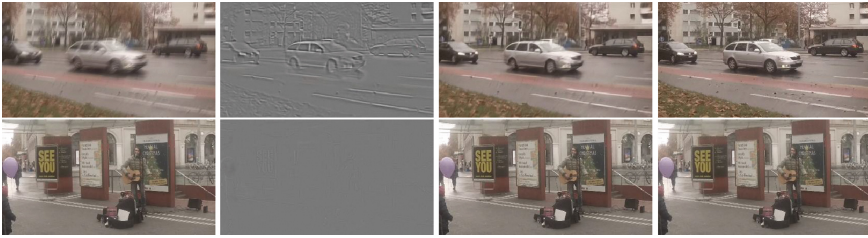
Fig. 10. The images with highest (first row) and lowest (second row) residual norm in the output layer. The image in the first column is the input, the second column shows the estimated residual (the network output), the third column is the deblurred image (first column + second column), and finally the forth column is the ground truth.
