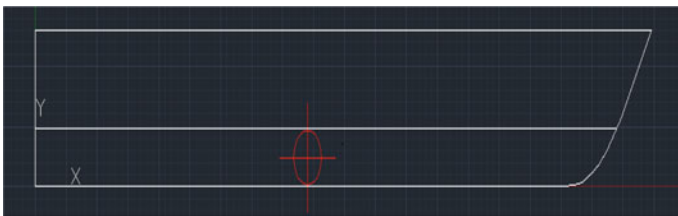
Fig. 12 Position of the anode on the hull
