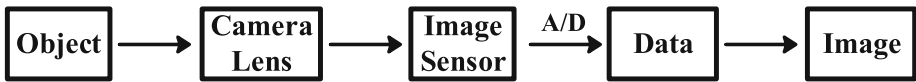
Fig. 1. Procedure of taking photo with camera: the data is YUV format and the image is JPEG format.
