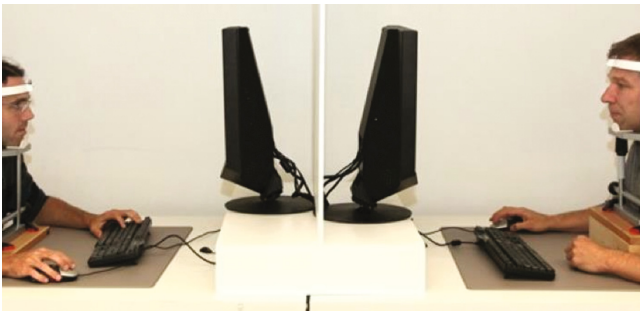
Fig. 1. The setup for the dual eye-tracking experiments, where the participants are separated by a wooden wall. They could not see each other, but they were asked to discuss with each other and the two screens were completely synchronized.
