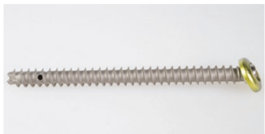
Fig. 12.5 Specifically designed cannulated, fully threaded screw with fixed washer. The tip of the screw is perforated laterally at different sites to achieve even cement distribution. For better anchorage in osteoporotic bone, the surface of the screw is roughened
