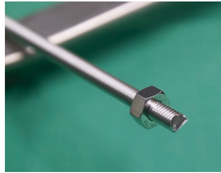
Fig. 13.8 Cutting the bar with the side cutter causes a plastic deformation of the bar end making removal of the bar later on difficult
