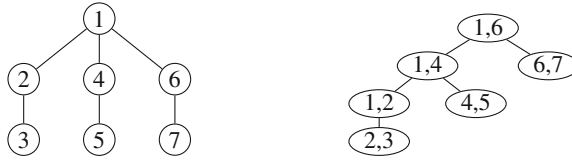
Fig. 1. A graph G (left) and an optimal (special) tree decomposition \mathcal{T} = (T, \chi) of G (right).
