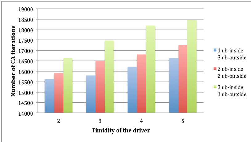
Fig. 8. The impact of the number of unloading-inside bays and unloading-outside bays and timidity of the driver on the number of iterations of cellular automaton [own study]
