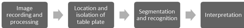
Fig. 2. Flow diagram illustrating operation of the actual system for recognizing license plates [own study]
