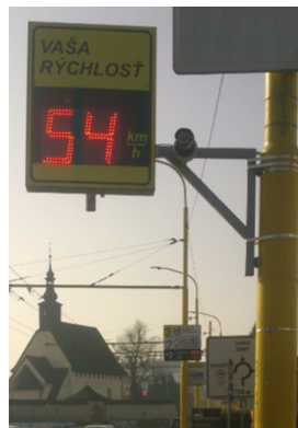
Fig. 2. Speed measuring device GEM CDU 2605 Zeus [own study]
