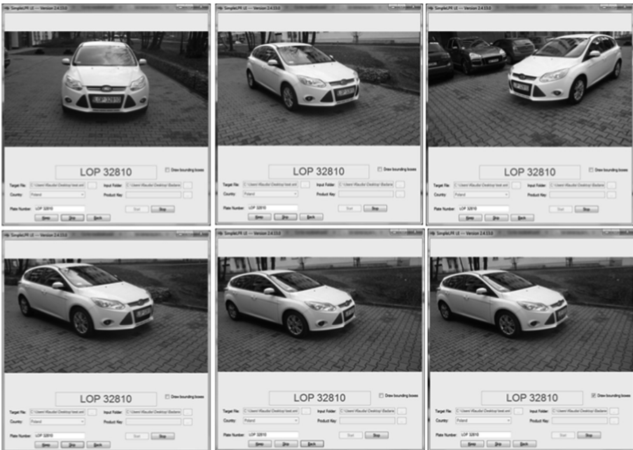
Fig. 7. The effect of pictures taken at various angles on ALPR [own study]
