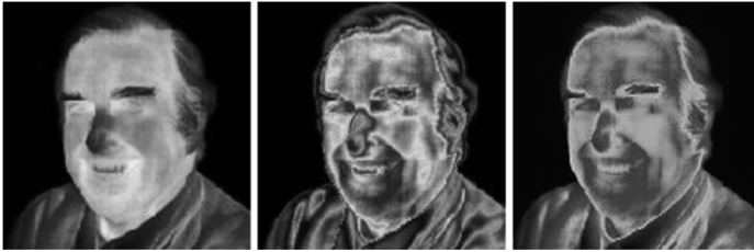
Fig. 4. Examples of different thermographic imaging effects depending on the temperature range applied: 25.4–35.7 °C, 25.4–36.6 °C, and 26–36.9 °C, respectively [27]
