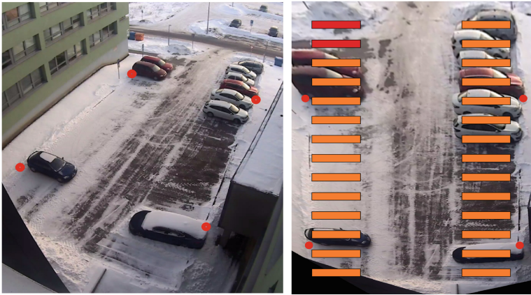
Fig. 7. Original (left) and transformed (right) image with displayed calibration points and detection zones [own study]
