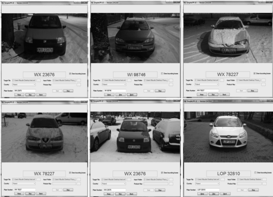
Fig. 6. Impact of light intensity (respectively 8 lx, 8 lx, 12 lx, 4672 lx, 5382 lx and 6998 lx) on ALPR quality and reliability [own study]
