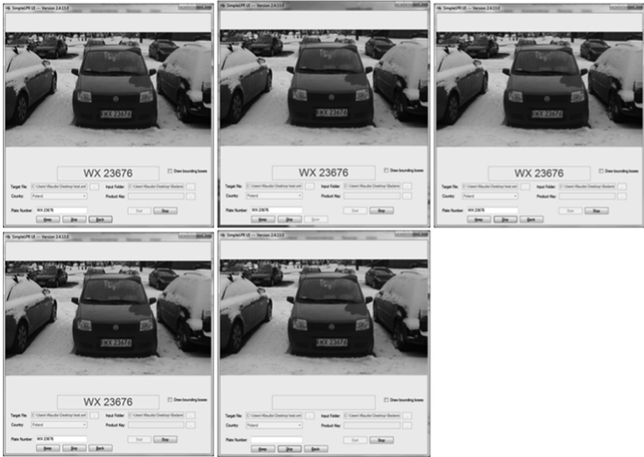
Fig. 8. The effect of image resolution on ALPR quality and reliability [own study]
