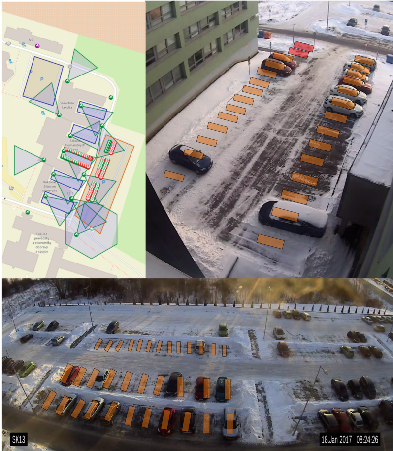
Fig. 6. Concept of the secured parking system in UNIZA campus [own study]
