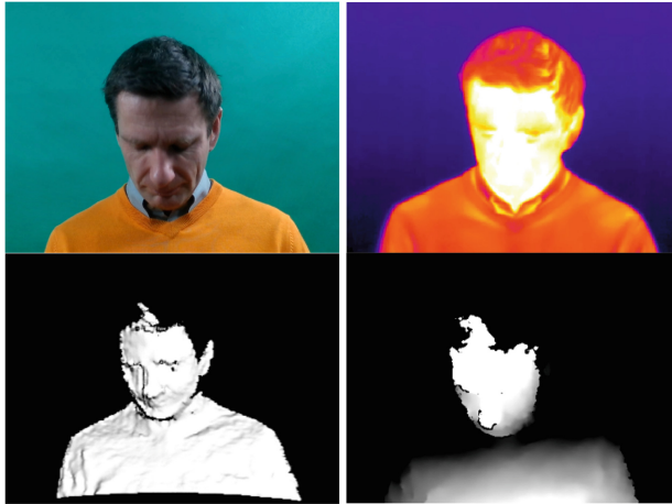
Fig. 8. Selected views of the driver's head and torso areas, visible, thermal (from LWIR), cloud of points and depth map (both from NIR).
