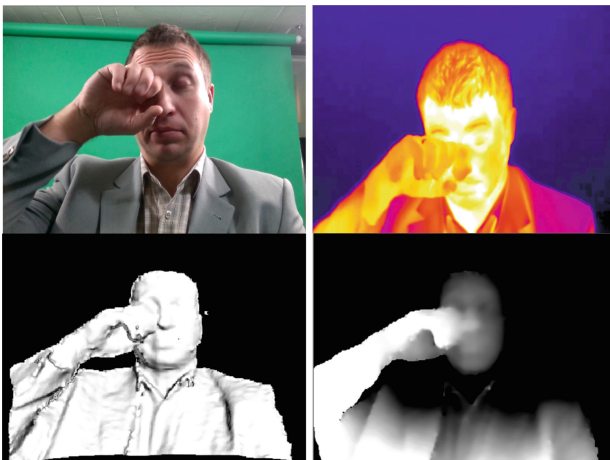
Fig. 7. Selected views of the drivers head and torso areas, visible, thermal (from LWIR), cloud of points and depth map (both from NIR).
