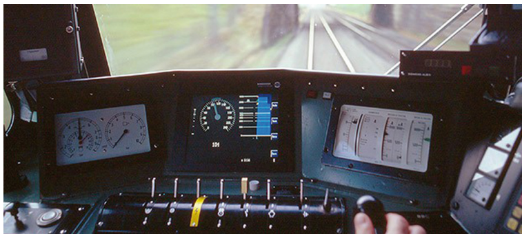
Fig. 6. Subsystems of the cab's signalization in the ERTMS/ETCS system [20]
