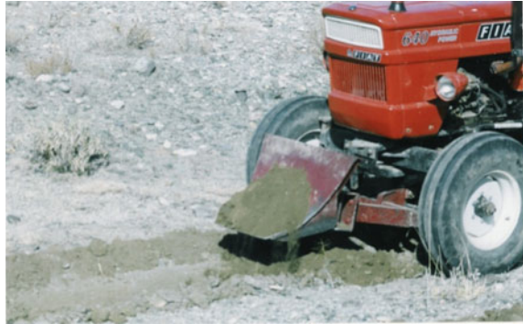
Fig. 6 Pit maker for making pits in ditches. Photograph Irfanullah Sahibzada
