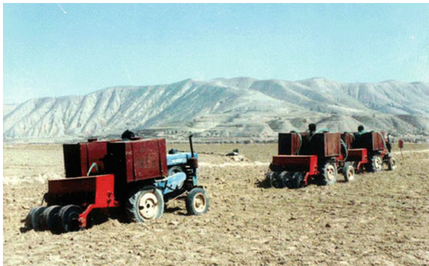
Fig. 7 An integrated machine with a water tank mounted on a sowing machine for supplying a small amount of water in the seeding ditch. Photo Li Yuanhong (2000)
