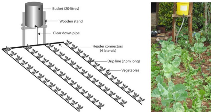
Fig. 5 Typical 20-litre low-head drip irrigation system mainly used for kitchen garden. Source Ngigi et al. (2005a)
