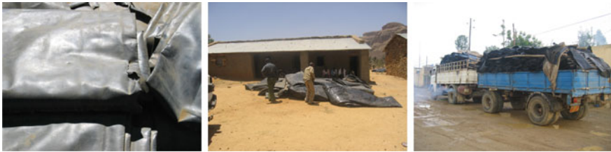
Fig. 11 Plastic liner damaged during transportation and storage. Location: Gulomekeda and Mekelle. Photograph : Gebremedhin Berhane
