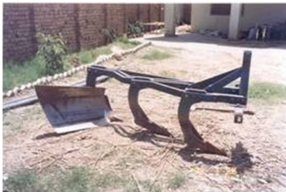
Fig. 5 Ditcher, specialized instrument for ditch making. Photograph Irfanullah Sahibzada
