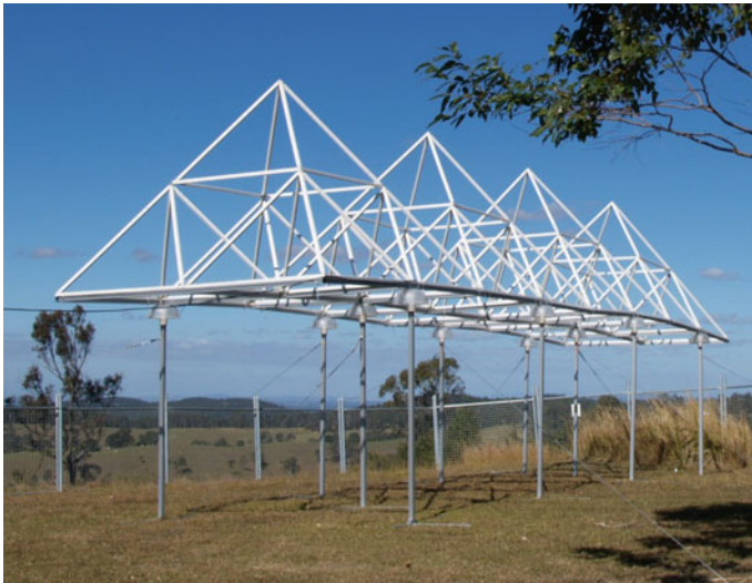
Fig. 8.13 Ion emitter used during earlier projects of WeatherTec-Services GmbH in 2007 in Queensland, Australia; the very thin wires can hardly be seen (Photo: Wilderer)
