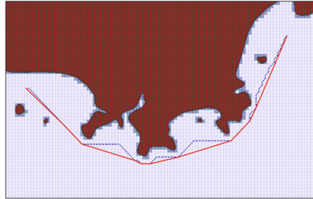
(a) the path planning results of the improved A* algorithm
