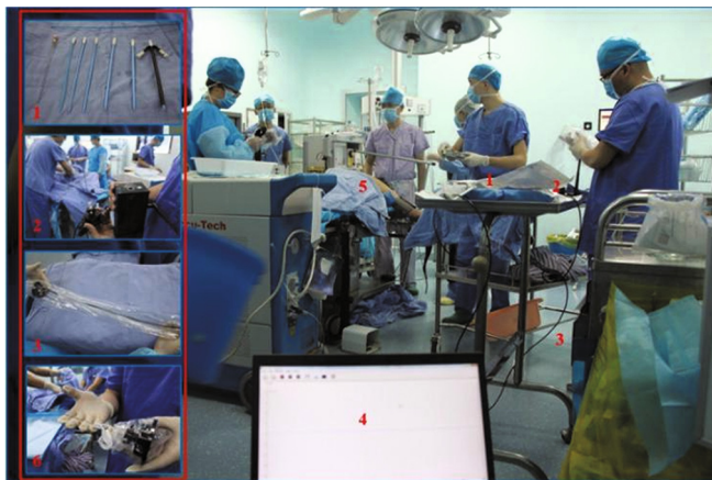
Fig. 2. Clinical trials setup: 1-Surgical instruments, 2-Force sensor and Connector, 3-Data conversion line, 4-Acquisition software, 5-Patient, 6-Puncture devices integration
