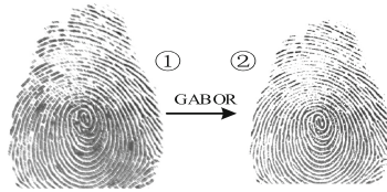
Fig. 5. Gabor filtering effect, (1) fingerprint samples, (2) filtering results
