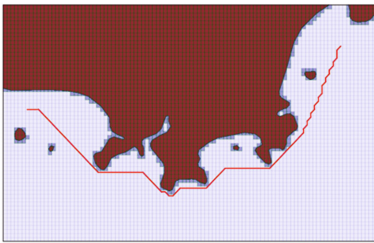
(a) the path planning results of the improved A* algorithm
