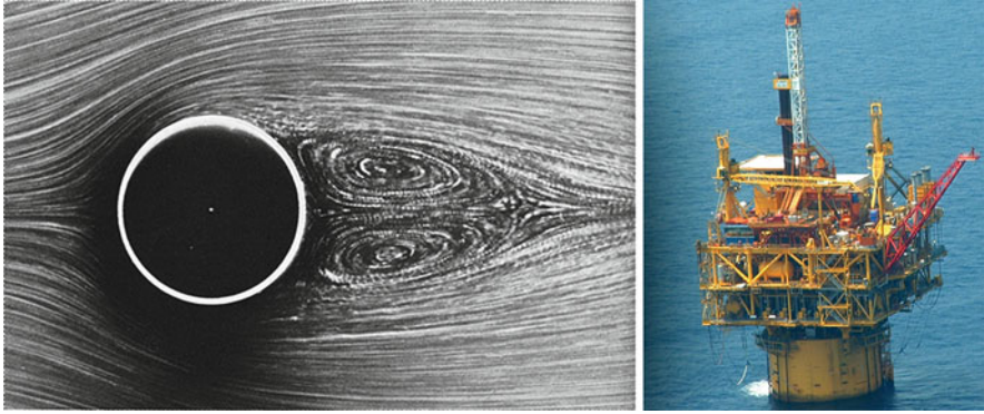
Fig. 1 (Left) Highly symmetric flow past a cylinder. (Right) An oil rig. Credit: VaderSS from Wikipedia
