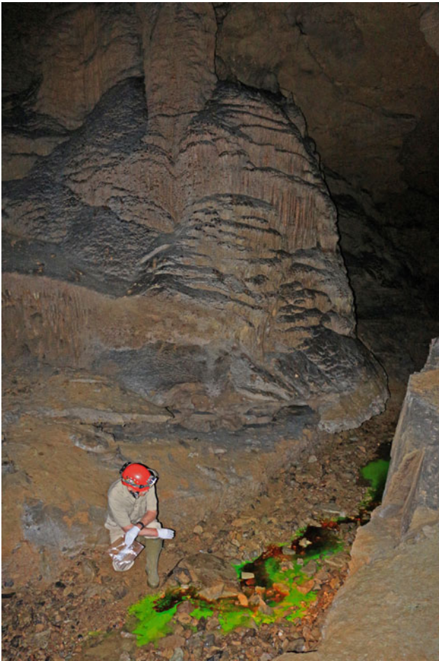
Fig. 3.32 Beginning the tracer test in McClung Cave that established the connection to Sweetwater River, the large stream passage in Maxwellton Cave, May, 2017. Photo by Clifford Lindsay. Used with permission
