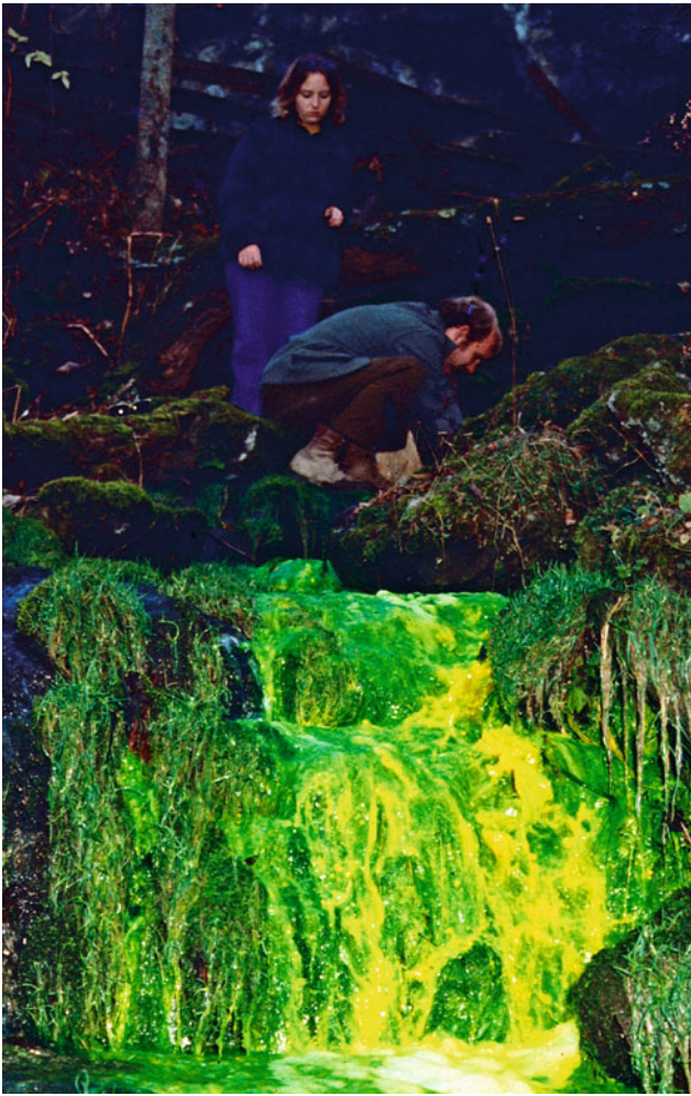
Fig. 3.5 Fluorescein sodium dye injected in the stream from Boyds Cave in Monroe County
