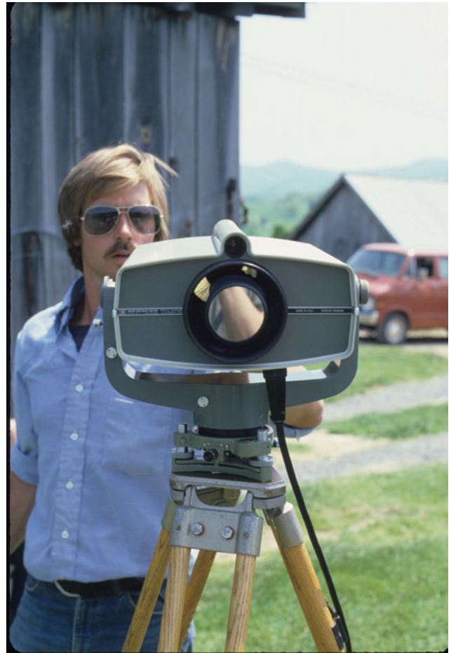
Fig. 13.8 Tommy Shifflett using an electronic distance meter (EDM). A theodolite and EDM were used to create an accurate surface survey
