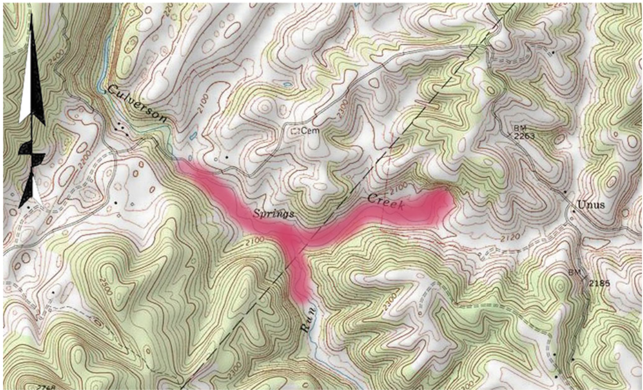
Fig. 10.3 Temporary lake is shown in red on this topographic map. The lake as shown here, is 1 mile in length. There have been flood events where the lake has extended much further up the blind valley
