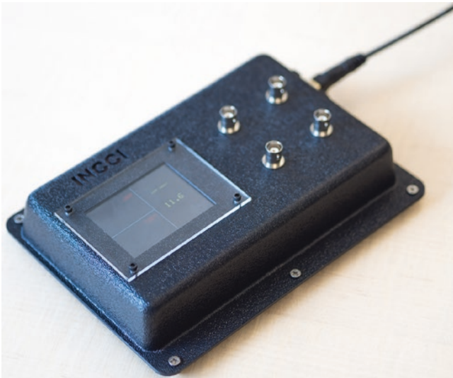
Fig. 1 The assembled device prototype for real-time noninvasive ICP estimation
