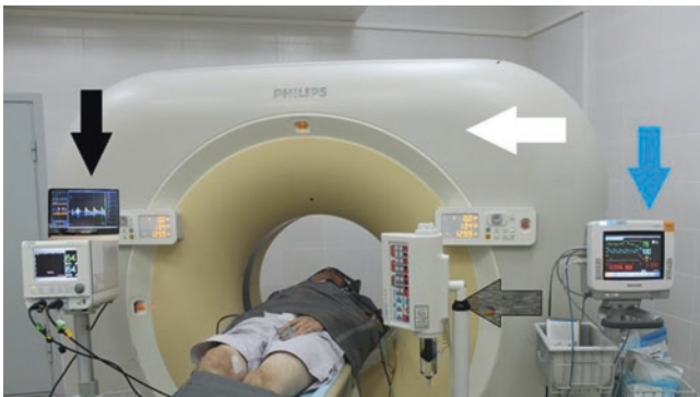
Fig. 1 The investigation system appearance. A white arrow indicates a computer tomograph, a black arrow shows a TCD, a blue arrow shows ECG-ABP monitor and a gray arrow marks a syringe-injector
