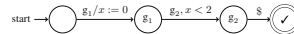
Fig. 13. GEAR . The set W (length 307–1,011,427) is generated by the automatic transmission system model in [16]. The pattern, from \phi_5^{AT} in [16], is for an event in which gear shift occurs too quickly (from the 1st to 2nd).
