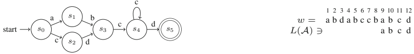
Fig. 4. Pattern matching. For the pattern NFA \mathcal{A} on the left, for which it is easy to see that L(\mathcal{A}) = L(\{\mathbf{ab}, \mathbf{cd}\} \mathbf{cc}^* \mathbf{d}) , the output is \{(9, 12)\} as shown on the right.
