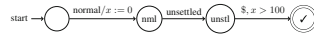
Fig. 12. SETTLING . The set W (length 472–47,200,000) is generated by the Simulink powertrain model in [17]. The pattern (Requirement (32) in [17]) is for an event in which the system remains unsettled for 100 s after moving to the normal mode.
