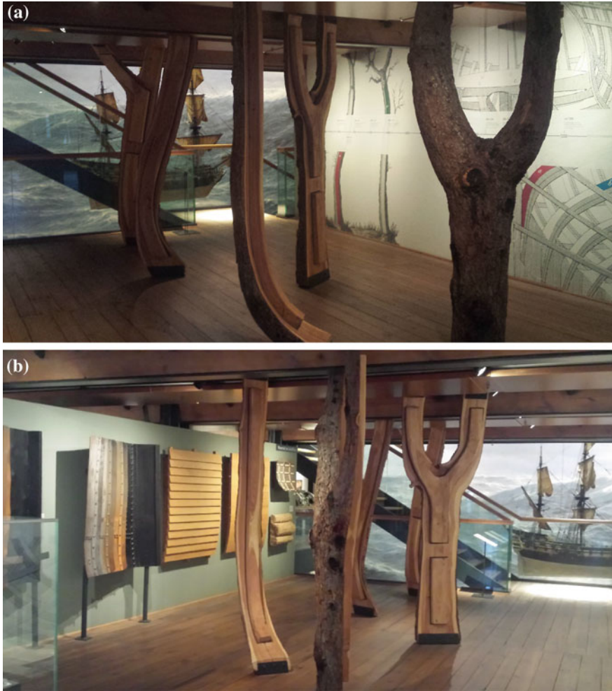
Fig. 3.5 Exposure in the International Maritime Museum in Hamburg illustrating the selection process of trees having a shape favourable for the building of ship rib structures. Photograph by the author, 2017
