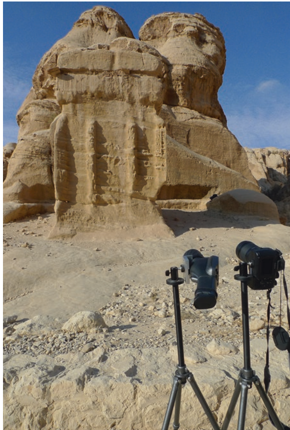
Fig. 5.3 Data acquisition on site with thermal infrared sensor ( left ), and visible/near-infrared camera
