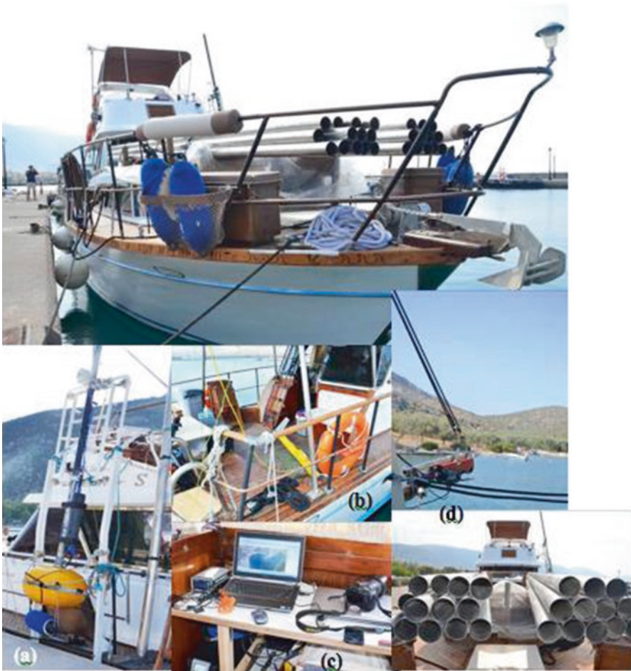
Fig. 9.71 The vessel “MY LORD, MY LADY” which was used for the remote sensing survey and the sediment sampling, equipped with (a) the sub-bottom profiler (over the side), (b) the side-scan sonar, (c) acquisition unit, and (d) sampling devices (Photo courtesy G. Papatheodorou, University of Patras)
