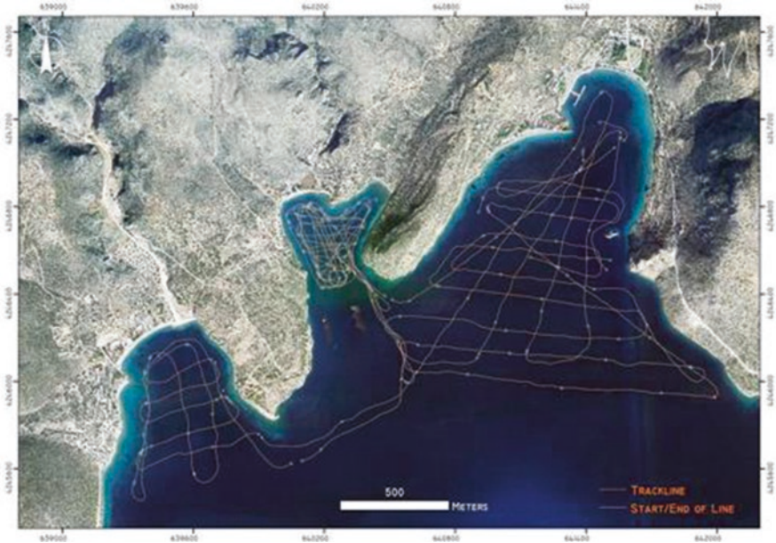
Fig. 9.74 Map of the surveyed areas showing the tracklines of the side-scan sonar and sub-bottom profiling. From right to left – Ag. Isidoros, Potami/Ag. Sotirios, and Valtos (Photo courtesy G. Papatheodorou, University of Patras)
