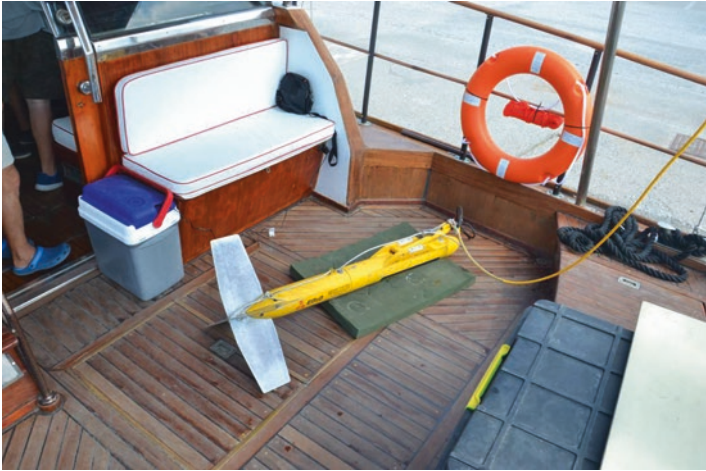
Fig. 9.72 Dual frequency towfish 272TD with the Kevlar-type cable
