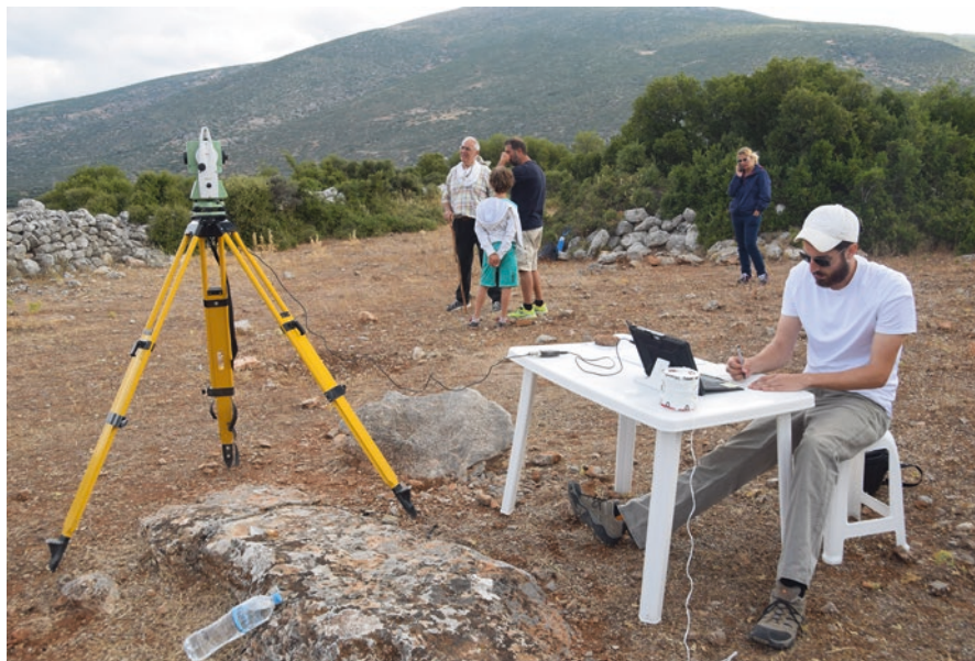
Fig. 9.5 For geodetic measurements, a TopCon GPT 3003 total station was employed. For daily excavation recording, a Leica TS02 Reflectorless Total Station was used
