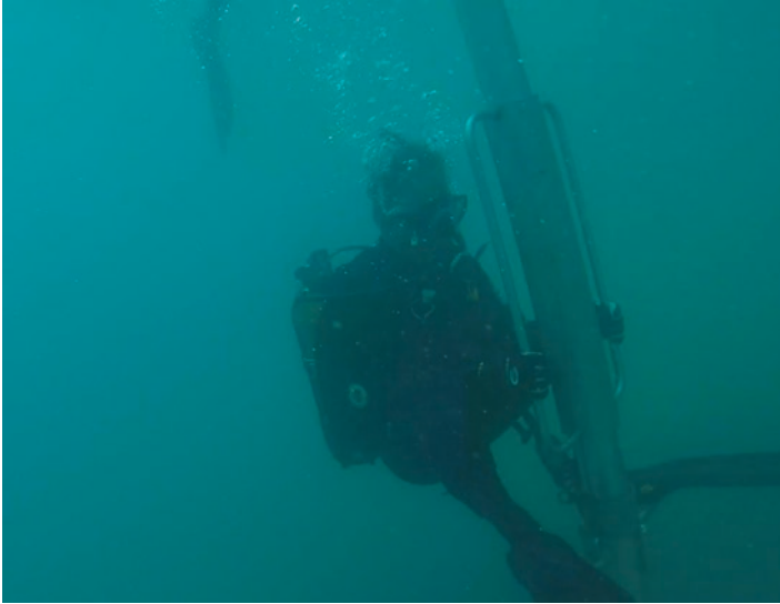
Fig. 9.80 Thomas Levy using hammer core system in Potami Bay. The hammer has two handles on the hammer, which is raised by the diver and released to hammer down the core barrel (Photo – Richard Norris, Scripps Institution of Oceanography, UC San Diego)
