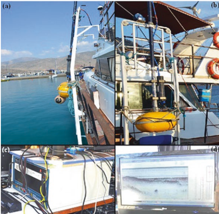
Fig. 9.77 (a, b) O.R.E. Model 132A/132B over-the-side Transducer Mounting (c) Universal Transceiver of the chirp system and (d) a chirp seismic profile collected from the surveyed area (Photo courtesy G. Papatheodorou, University of Patras)
