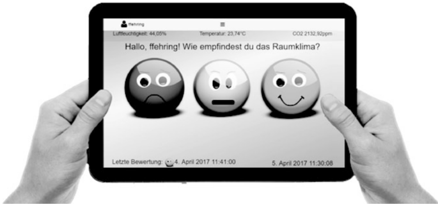
Fig. 4 Visual display unit with visualization of air quality measurement and Feedback buttons
