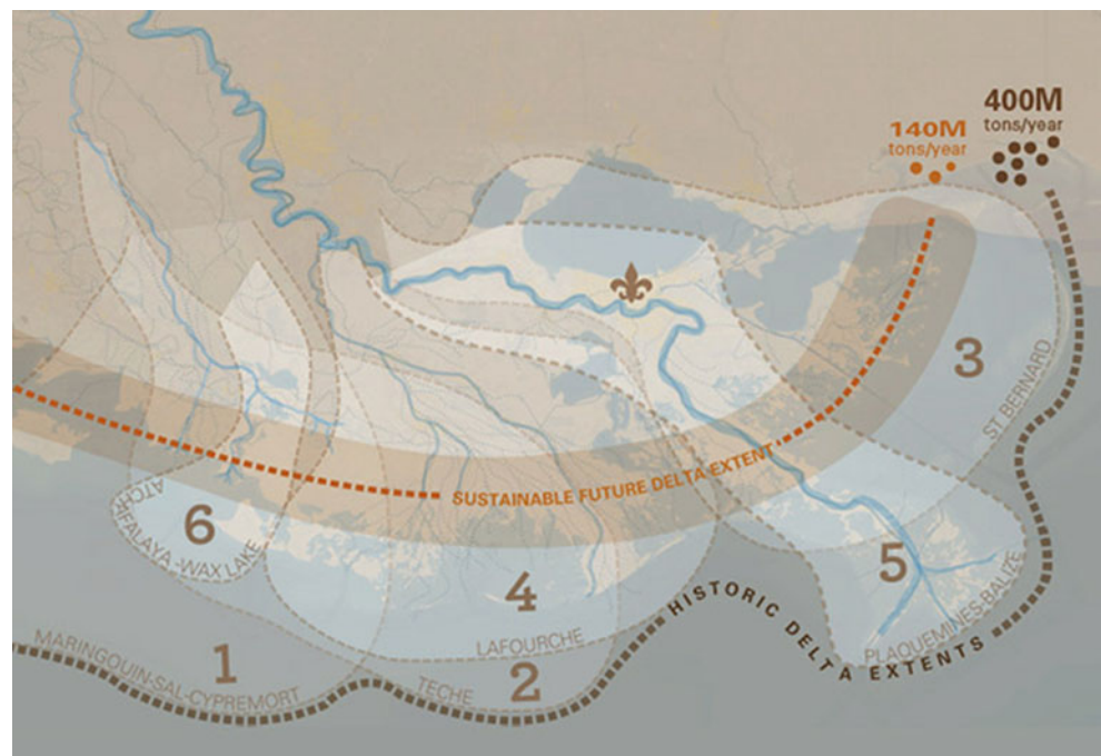
Fig. 3 Less land is sustainable today, compared to when the MRD was built, due to reduced sediment loads in the Mississippi River (The Baird Team 2015)
