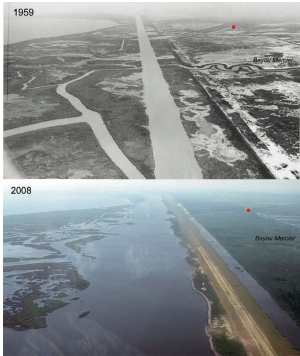
Fig. 10 Widening of the MRGO channel from 1959 to 2008 near Bayou Mercier. Red dot marks the same location in both photographs (from Shaffer et al. 2009b)
