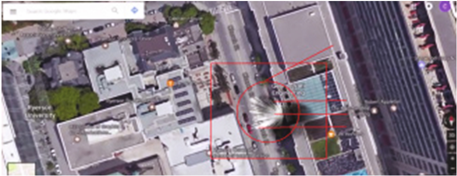
Fig. 1. UAV Guided IED Explosion Simulation, the simulation uses a DFC model where shrapnel is considered as an explosive dispersal of solid particles.
