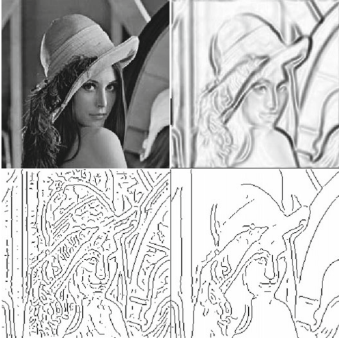
Fig. 3.48 Wavelet analysis of an image ( top left ). Top right Modulus of the wavelet transform. Bottom left Maxima of the modulus. Bottom right Thresholded maxima. From Stéphane Mallat
