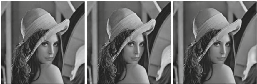
Fig. 3.49 Reconstruction of the image in Fig. 3.48 by inverse wavelet transform. Left Original image. Centre Reconstruction from weakly thresholded maxima. Right Reconstruction from strongly thresholded maxima (compression by a factor of 32). The geometry of the image is perfectly preserved. Only the textures are slightly smoothed. From Stéphane Mallat
